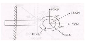
Q6.) A system of forces are acting on a body as shown in the below fig. Determine the magnitude and direction of the resultant.
