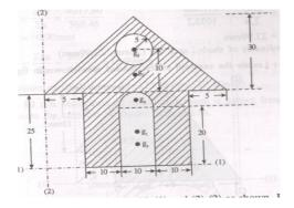
**Q23.)** A semicircle of diameter 100m is cut out from a quarter circle of radius 100mm. Locate the centroid of the shaded area as shown in the below fig.
