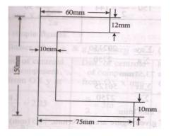
Q22.) Locate the centroid of the shaded area as shown in the below fig
