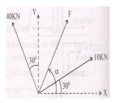
Q29.) Find the value of resultant of the system of forces as shown in the below fig.
