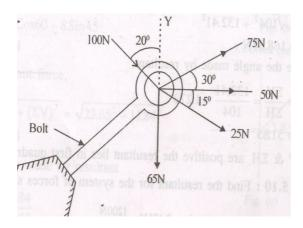
**Q29.)** A system of forces are acting on a body as shown in the below fig. Determine the magnitude and direction of the resultant.
